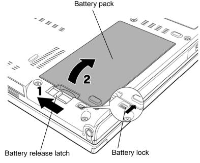
Figure 4-1 Removing the battery pack
